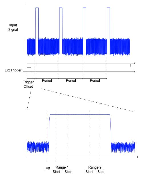
The gate ranges define the part of the I/Q capture data taken into account for the statistics calculation. These ranges are defined relative to a reference point T=0. The gate interval is repeated every period time until the end of the I/Q capture buffer.
