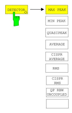
The *DETECTOR* softkey opens a submenu to select the detector and combinations of detectors.
