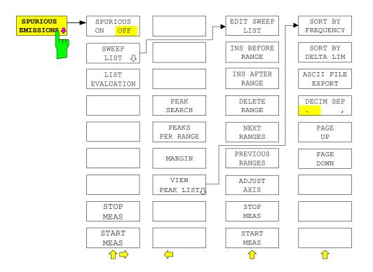
In the Spurious Emissions mode, the analyzer performs measurements in predefined frequency ranges with settings that can be specified individually for each of these ranges.
