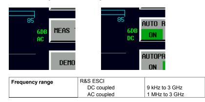
Measurements outside the valid frequency range are marked with the AC label in red
